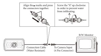
B. Run the cable from the camera to the monitor.
